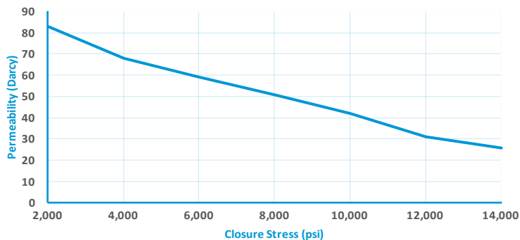
2 lb/ft 2 , 250°F, 2% KCl & Ohio Sandstone
